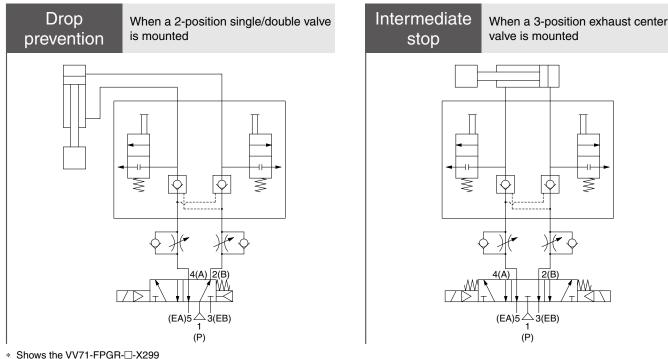
\* When single and double solenoid valves are used in combination, the SUP residual pressure release is intended to prevent cylinder dropping.
