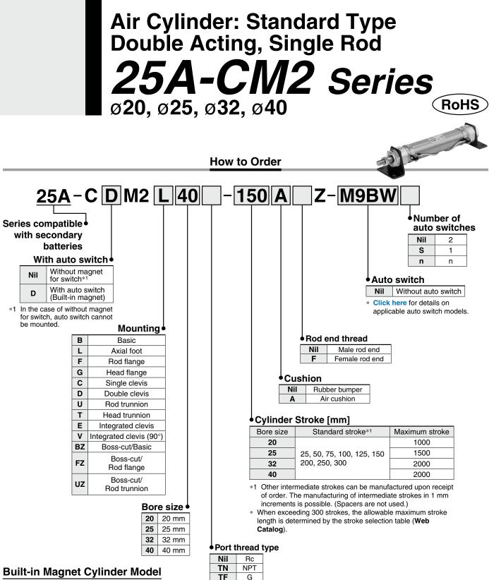
If a built-in magnet cylinder without an auto switch is required, there is no need to enter the symbol for the auto switch. (Example) 25A-CDM2F32-100AZ
