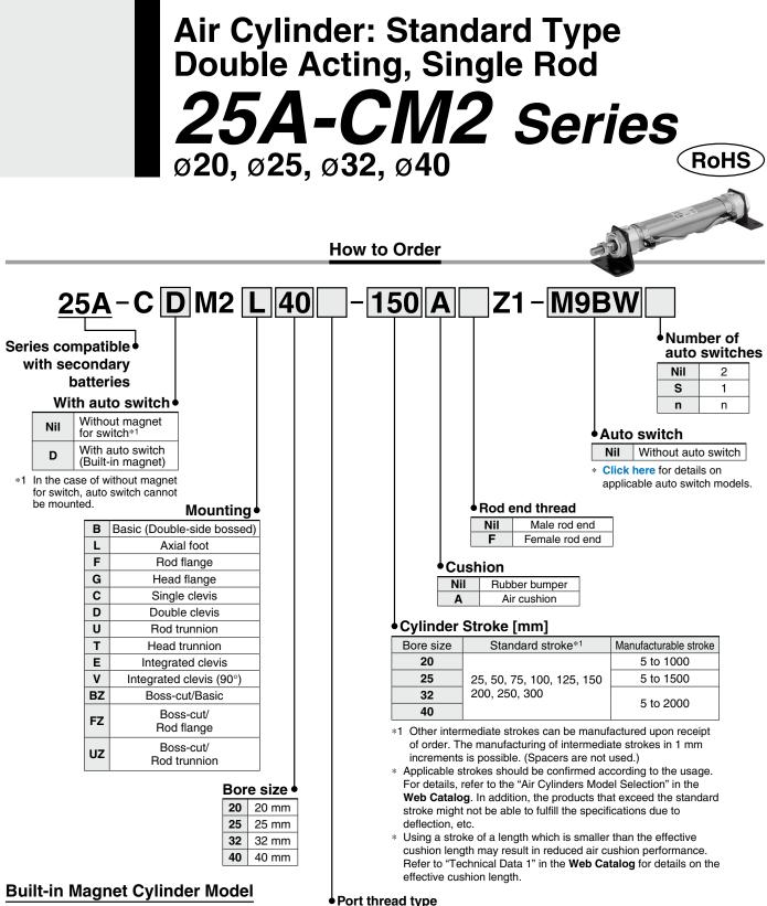
If a built-in magnet cylinder without an auto switch is required, there is no need to enter the symbol for the auto switch. (Example) 25A-CDM2F32-100AZ1
