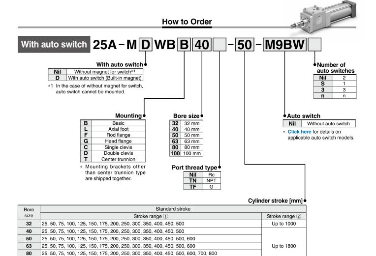
\* The manufacturing of intermediate strokes is possible. (Spacers are not used.)
